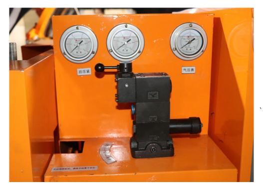
The hand valve for hydraulic clamp
