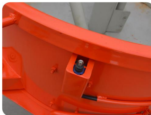
Limit switch for protecting operator
