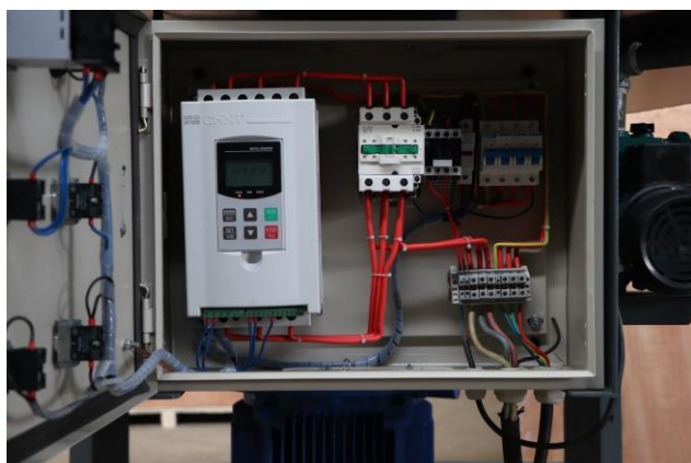
Soft start device, protect electric motor
