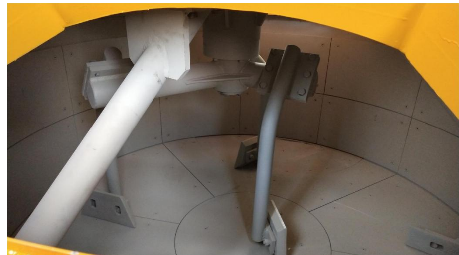
Cr-hard alloy cast iron liner and mixing blade.
