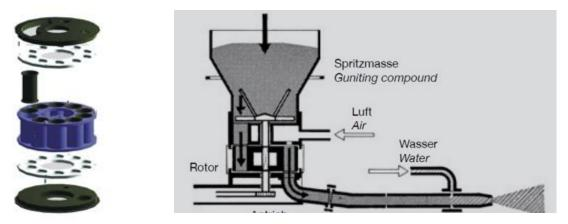
★ Rotor system could change different size rotor body, achieve different output capacity from 0.7m3/h to 3m3/h.
