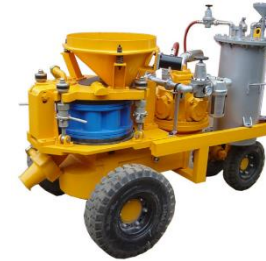
LSZ3000A air motor drive wet shotcrete machine
