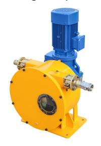
When the rotor unit drives single roller to rotate, hose is squeezed and deformed. After the roller rotate, the deformed hose recover by its elasticity. Thus the negative pressure in this hose is generated, sucking slurries, and discharging through output under rollers' push, finally forms pressure conveying of slurries.
