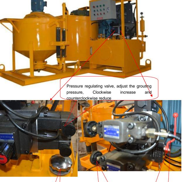
Speed control valve, Adjust the grouting displacement, Clockwise reduce and counterclockwise increase Oil adding part Relief valve, it is set well in the factory and do not turn.
