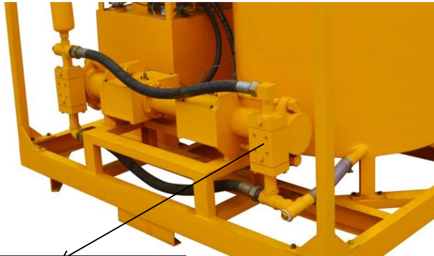
Newest design and easily to replace the piston
