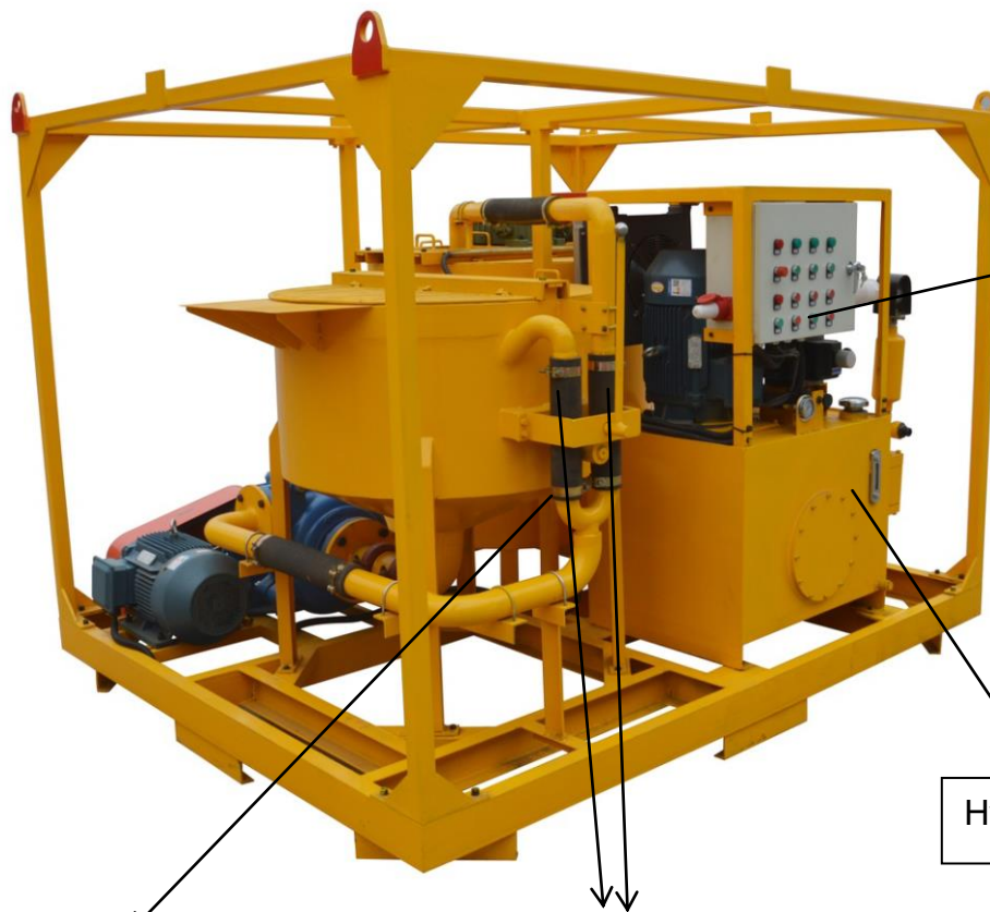
Special squeeze hose (resistant to more than 50000 times extrusion), no valve switch device
