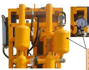
Double-Plunger plus two pulsation damper, even in 5MPa, the flow pressure surge is kept in low
