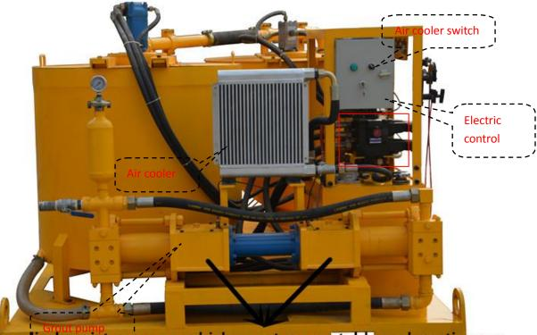
Double cylinder-piston pump which grout more stable and continuous
