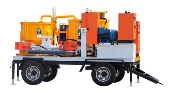
LGP400/1000/95/165DPL-E/A Fully automatic mobile grouting plant are integrated with a screw feeder, mixing, agitator and horizontal hydraulic pump. It is mainly used to be made such as cement slurry or bentonite slurry, etc., for injecting in the sub-soil for soil consolidation, piling or even for long transport of material.
