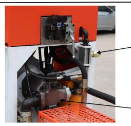
Adjustable output with this valve (LS control)
