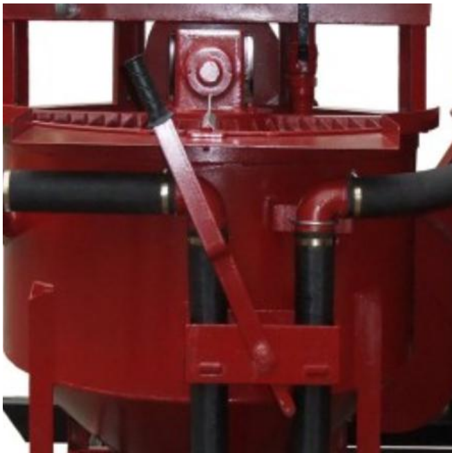
Recirculate/ Discharge system
